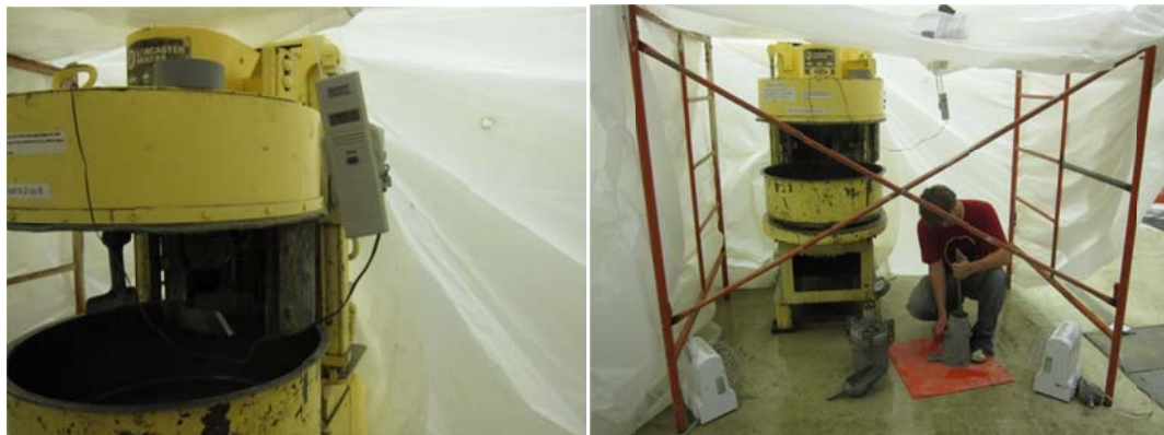
Figure 22. Testing set-up used for the high temperature extending mixing procedure: pan mixer and air temperature sensor control system (left) , enclosed testing area around mixture showing space heaters and fresh concrete test equipment (right).
