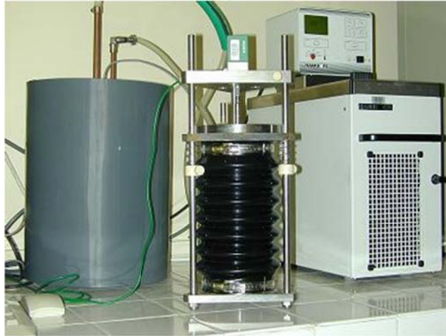
Figure 30. Test rig for monitoring Autogenous shrinkage in concretes.
