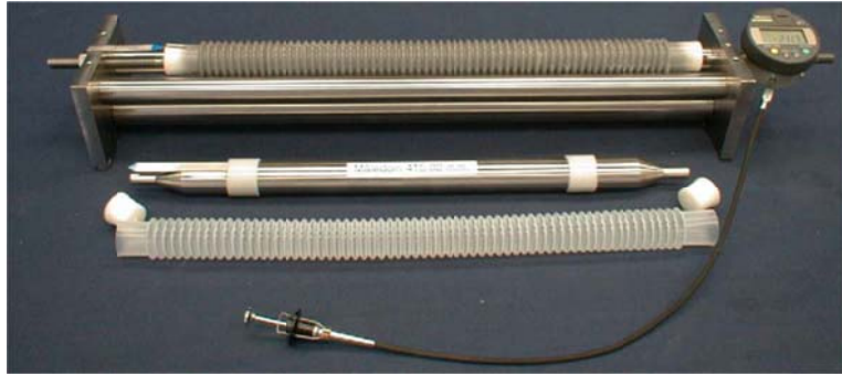
Figure 28. Auto-Shrink digital dilatometer by Jensen and Hansen [1995].
