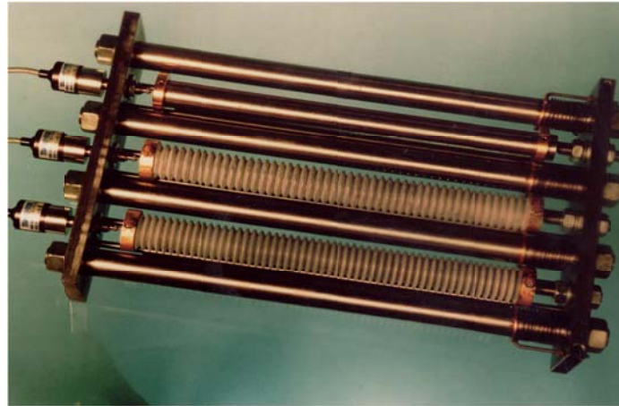
Figure 29. Auto-Shrink digital dilatometer for two specimens [1995].
