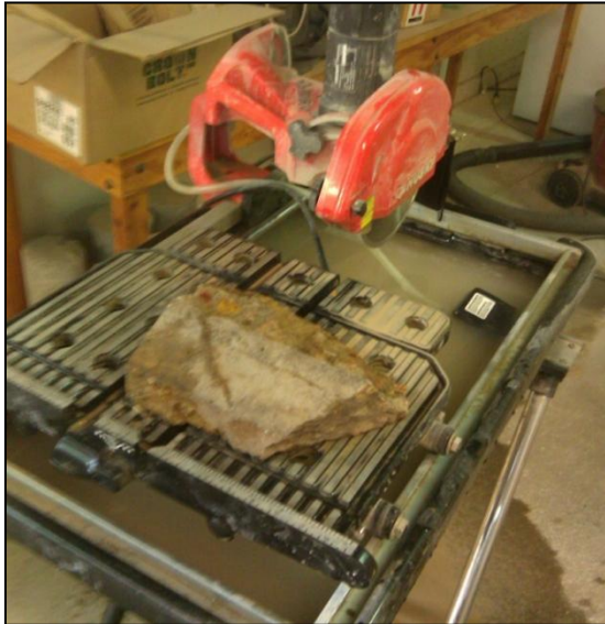
Figure 3.2 Cutting the 2” cubes.
