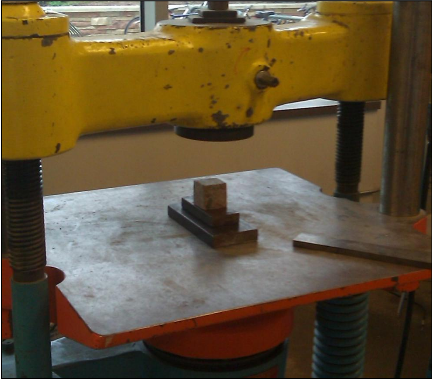
Figure 3.4 Compression test of the 2"x 2" concrete cube.
