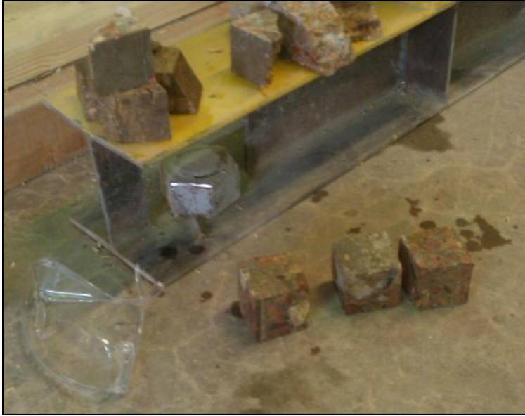
Figure 3.3 Three concrete cubes for testing.
