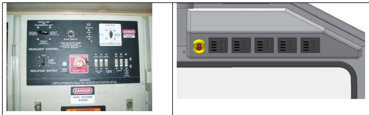
Figure 8. Existing Locomotive Rear Wall Engine Control Panel vs. NGLC Overhead Panel Design
