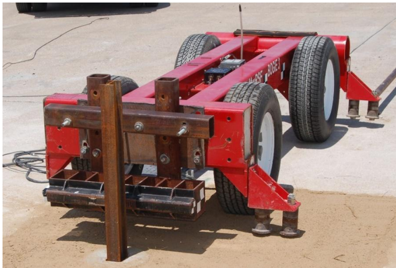
Figure 4.1 Rigid Frame Bogie with Impact Head
