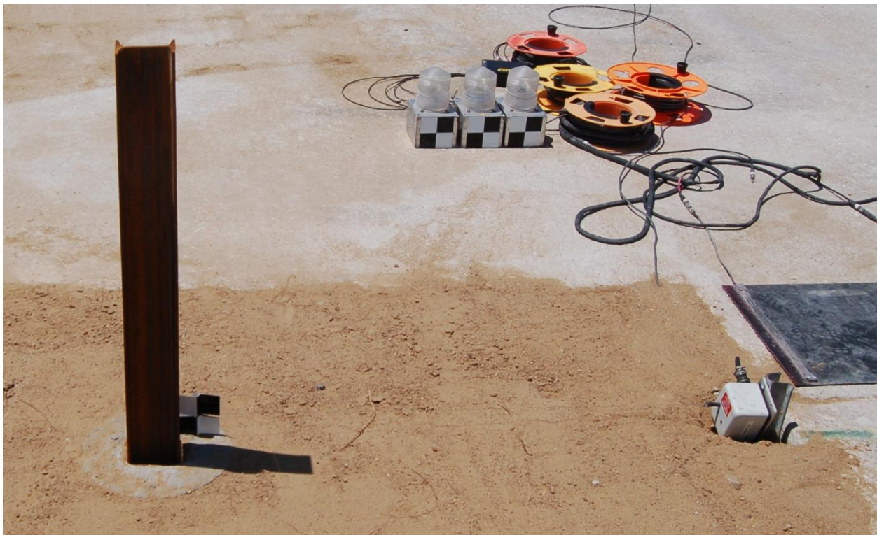
Figure 4.2 Typical String Potentiometer Setup
