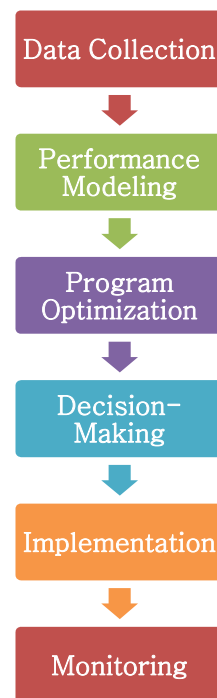
Figure 0-2 Basic Elements of Infrastructure Asset Management
