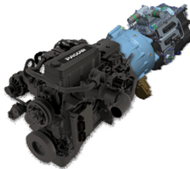
Figure 3-13. Image of Peterbilt/Eaton hybrid electric drivetrain.
