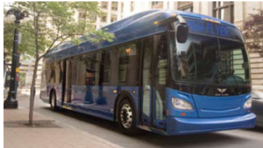
Figure 3-8. Image of New Flyer/Allison hybrid electric bus.
