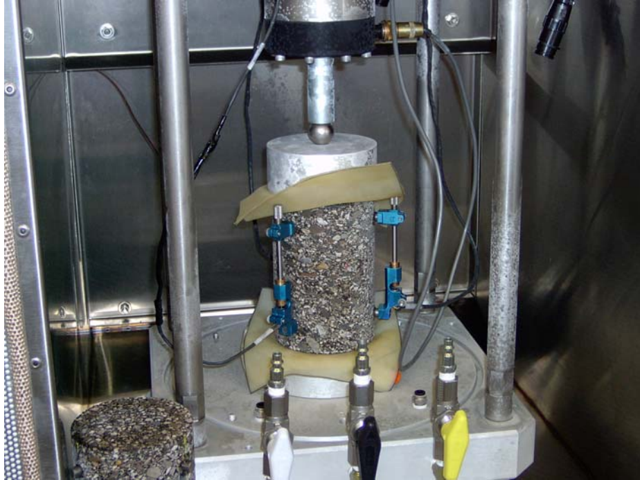
Figure 11 HMA sample ready for dynamic modulus testing.
