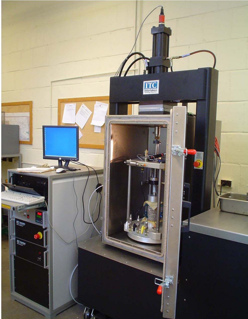
Figure 8 OSU's ITC dynamic modulus testing machine.
