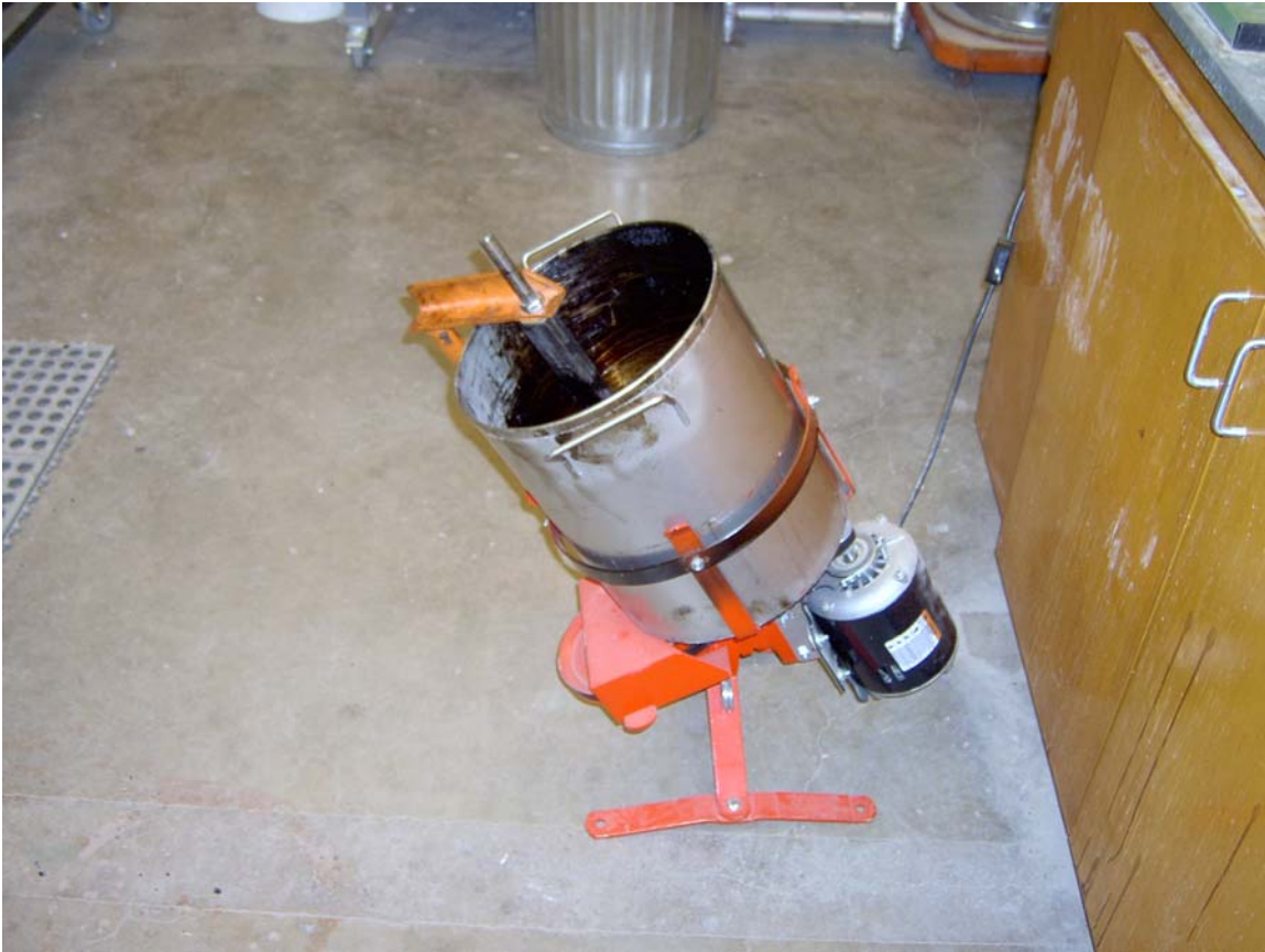
Figure 3 Bucket mixer used for mixing HMA samples.
