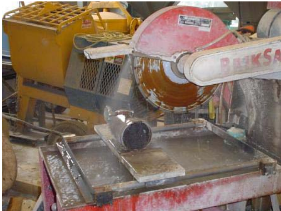
FIGURE 23 Sample is sawed to obtain parallel faces.
