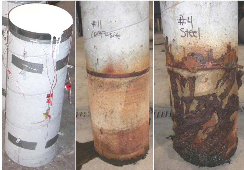
Figure 2.6: Condition comparison: (a) Typical control specimen (b) Typical hybrid corrosion specimen (c) Typical steel corrosion specimens
