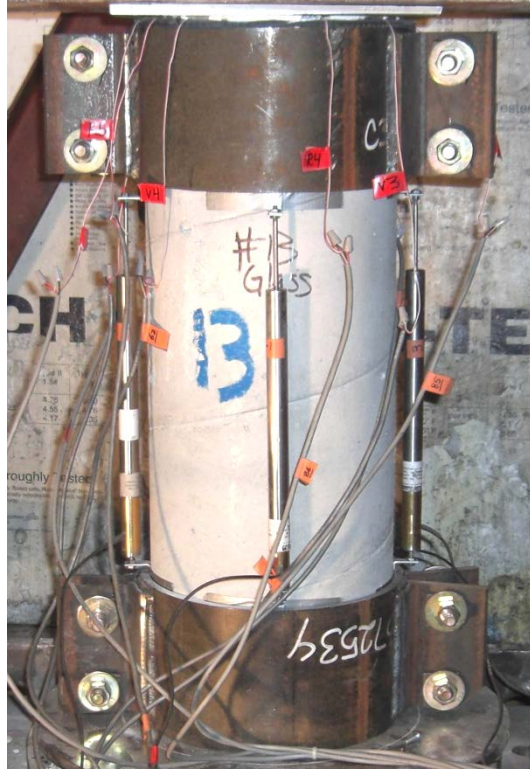
Figure 2.11: LVDT placement and steel confinement collars
