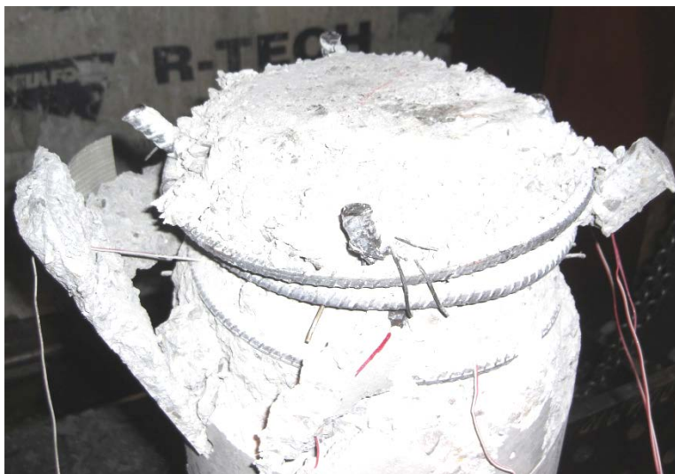
Figure 3.5: #1SCTL premature end crushing
