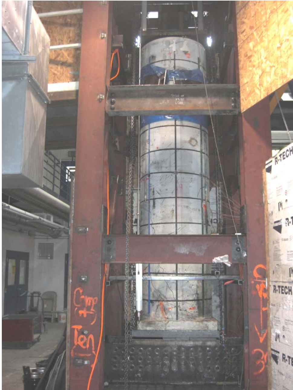
Figure 4.1: Column in load frame
