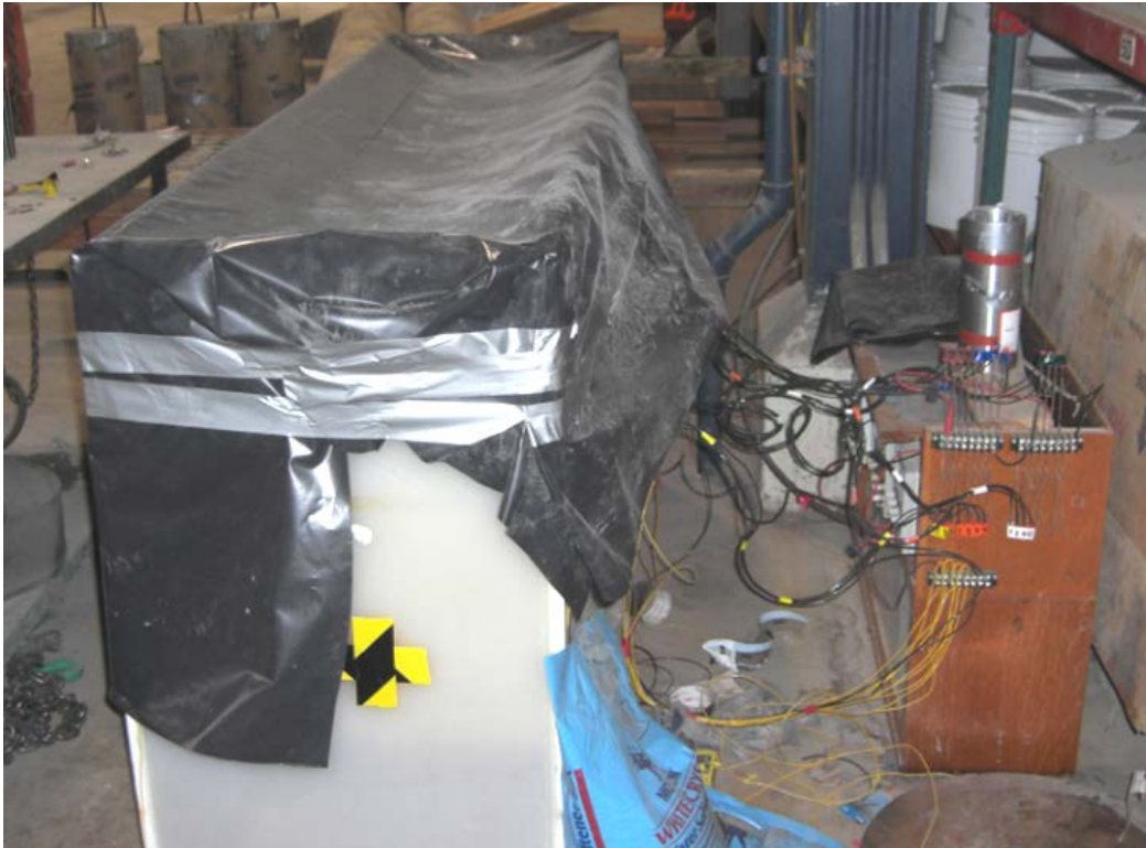
Figure 2.8: Corrosion system for medium-scale RC columns
