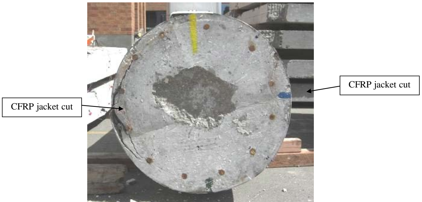
Figure 4.9: Picture of delamination of LG1 after testing
