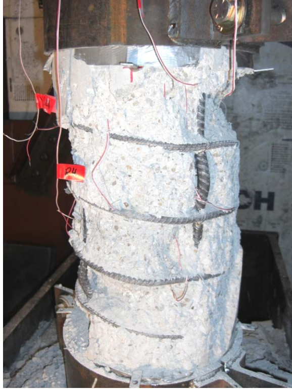
Figure 3.6: #2SCTL proper failure
