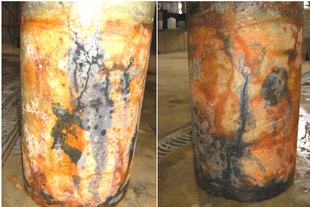
Figure 2.7: Trial corrosion specimen comparison (a) #7SCOREX after 5 weeks of corrosion (b) #8SCOREX after 10 weeks of corrosion
