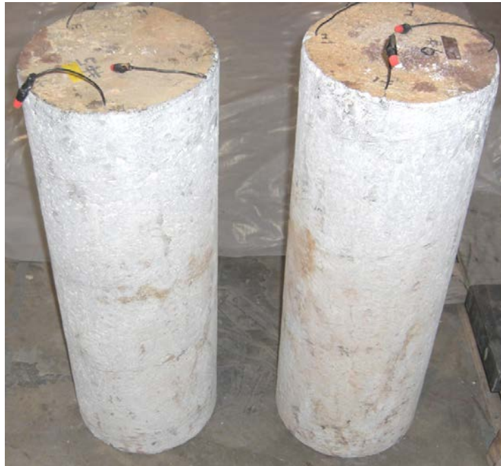
Figure 2.9: Roughened surface of Columns #5SCORW and #6SCORW
