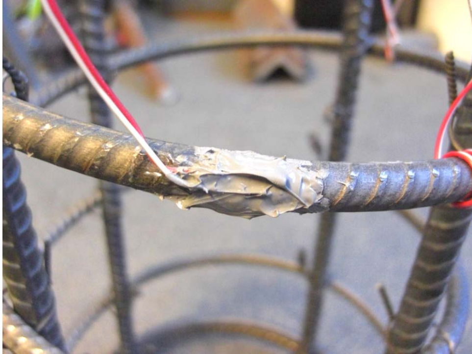
Figure 2.13: Internal strain gauge protective coating
