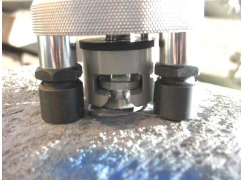
Figure 4.20: Elcometer Model 106 Adhesion Tester
