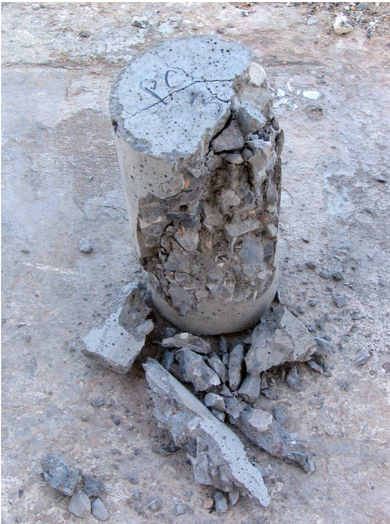
Figure 29: Plain concrete compression failure: brittle
