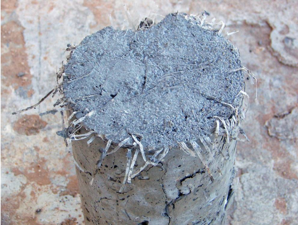
Figure 35: Concrete finish on Strux 90/40 high dosage mix after unmolding
