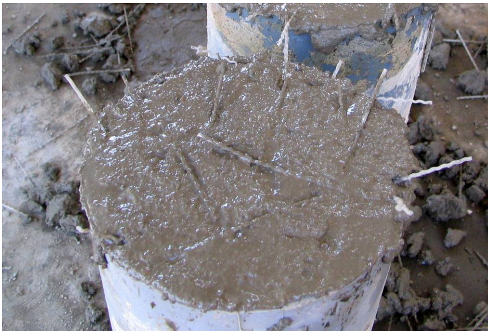
Figure 34: Concrete finish on HPP high dosage mix at time of casting
