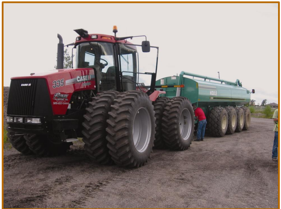
Large manure hauling tank on the MnROAD test track; fully loaded it weighs more than 134,000 lbs (distributed over four axles - not including the tractor).
