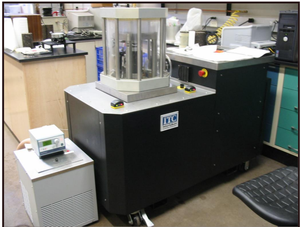
CIR-emulsion mixtures tested using an Interlaken Gyrotory Compactor Photo: Dr. Hosin "David" Lee, The University of Iowa/IIHR
