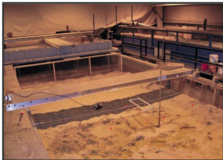
The water/sediment re-circulating flume for the RFID tests (antenna is at the center of the flume).
