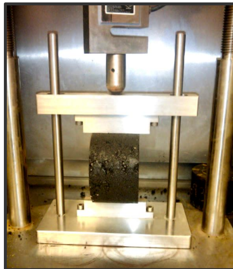
Indirect tensile strength test setup
