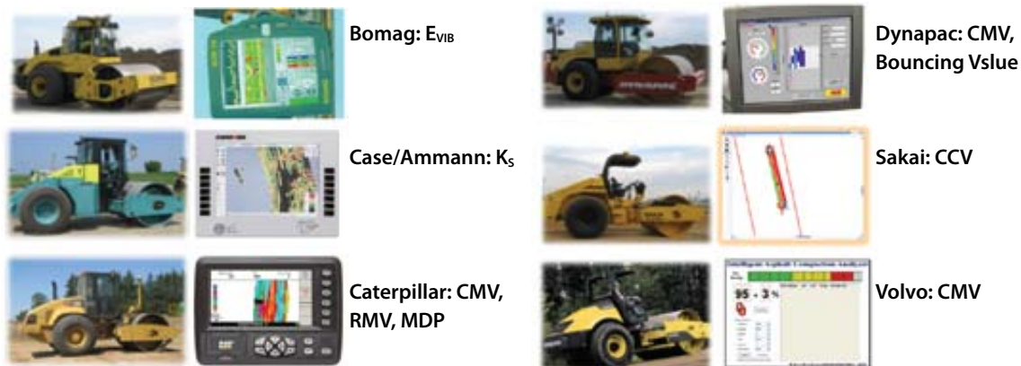
Figure 1. Smooth drum compaction monitoring systems for soil and aggregate.
