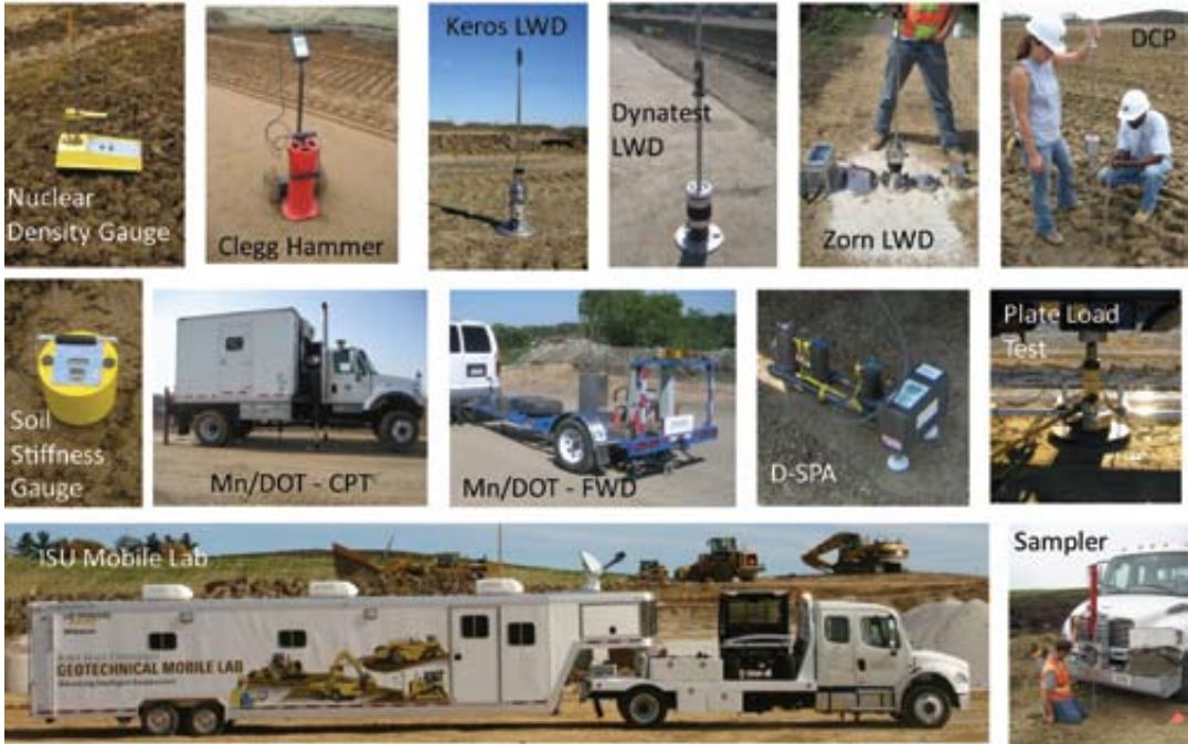
Figure 4. Various in situ compaction equipment for field QC/QA.
