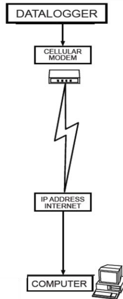
Figure 11 Communication between the datalogger (station) and the server
