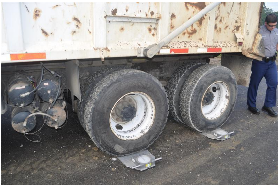
Figure 131 Portable scales used in weighing individual truck axles
