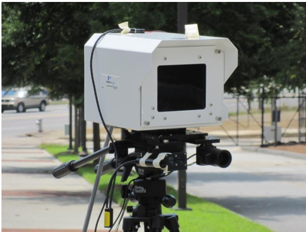
Figure 18 Initial System configuration IR illuminator t a laser trigger and camera.
