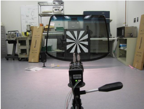
Figure 15 Transmission measurements at various orientations
