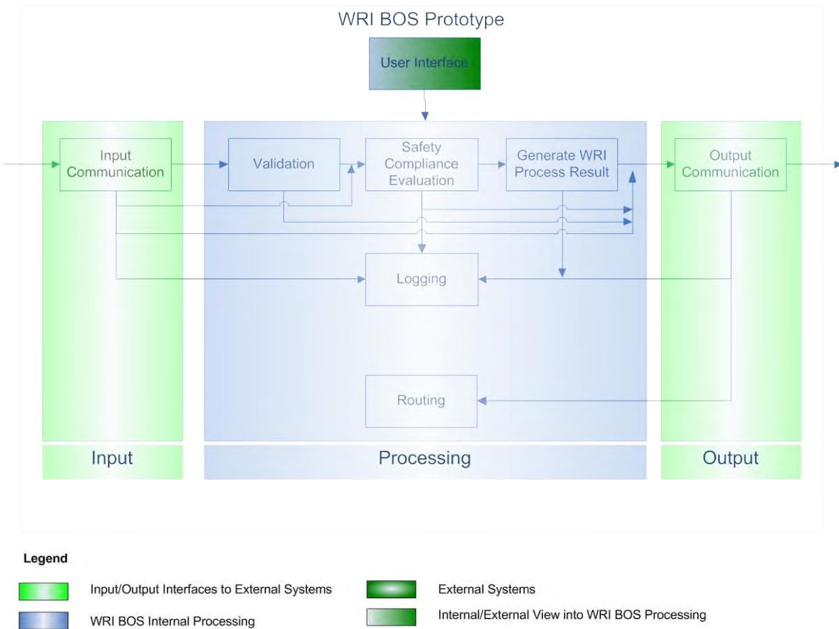
Figure 23. Diagram. GBOS communication and data processing flowchart.
