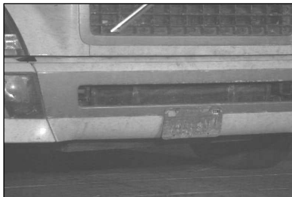
Figure 21. Photograph. Unreadable license plate from snow and ice accumulation.
