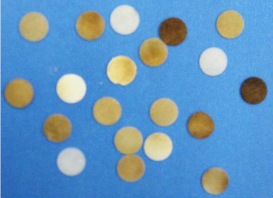
Figure 3. Pellets from various admixtures ready for IR scan
