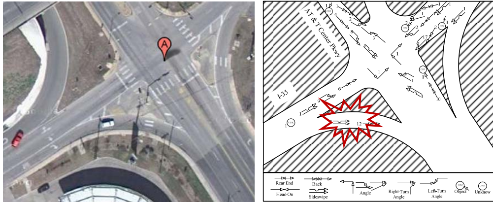
Figure 5-4: Rear-End Crash Hot Spots at AT&T Center Parkway at IH-35.
