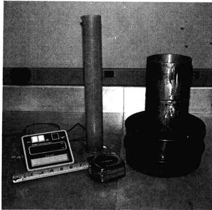
Figure 3.2: Apparatus for Constant Head Permeability Test
