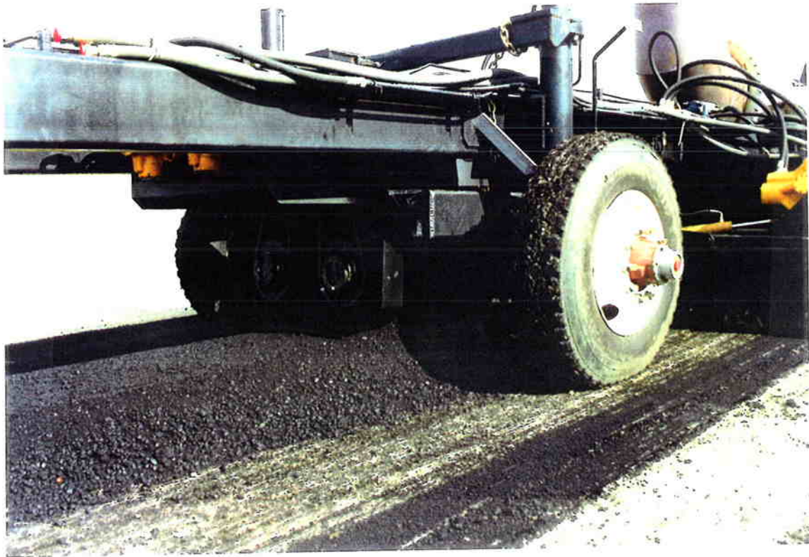
Figure 2.23 Close-up of pugmill at the rear of unit 3. (Photo courtesy of ARTEC.)
