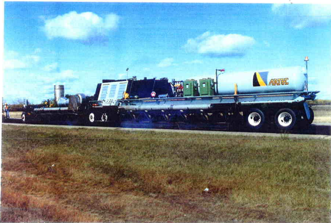
Figure 2.16 Artec multi-stage preheater (unit 1). (Courtesy, ARTEC)
