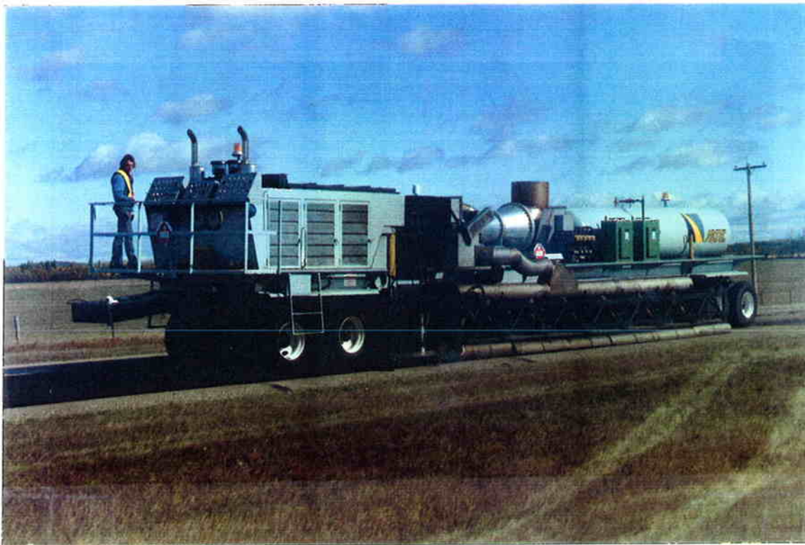
Figure 2.20 Close-up of Artec multi-stage first heater/miller (unit 2). (Photo courtesy of ARTEC.)
