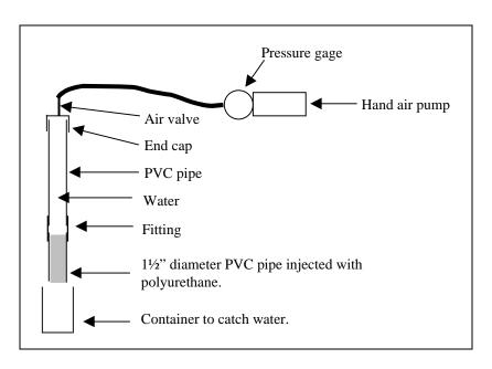
Figure 2.3: Apparatus to measure water permeability
