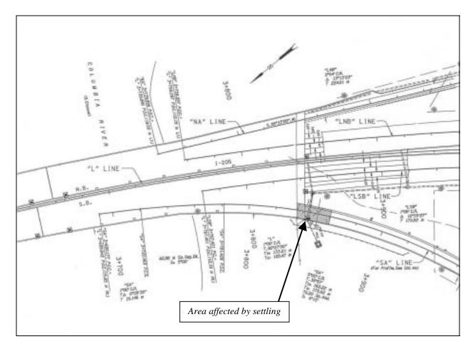
Figure 1.1: Location of slab jacking
