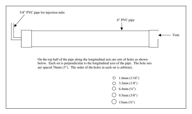
Figure 2.2: Fixture design for measuring invasiveness of injected polyurethane
