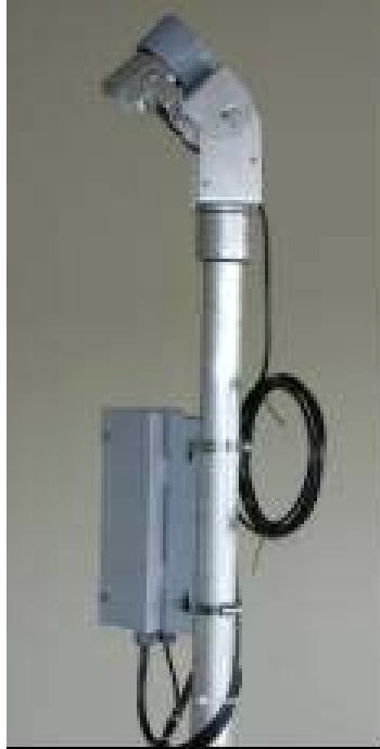
Figure 3.1: Laboratory set up of video camera and transmission equipment
