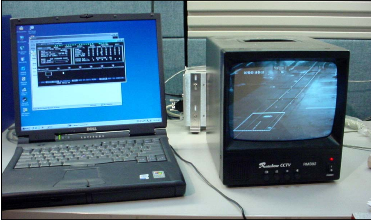
Figure 5.4: The microwave detection display (left) and the video detection display (right); a corner of the video detection module is also visible (center, behind the video monitor)
