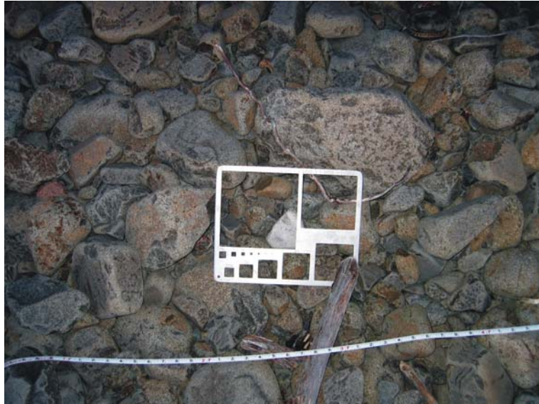
Figure 4.2: Example of a “gravelometer” being used at Neahkahnie to determine grain size statistics on the beach
