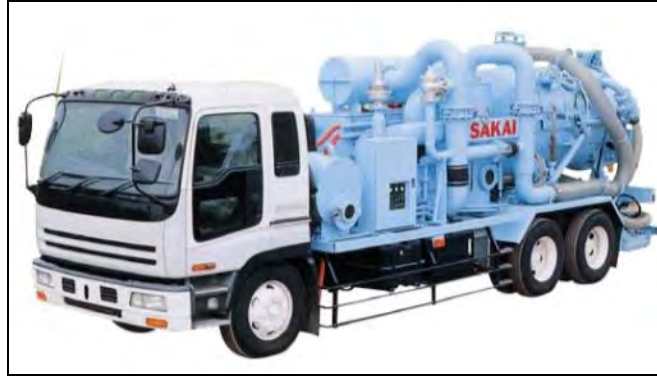
Figure 2.9: Sakai CH400-1 “Water drainage pavement restoration vehicle”
