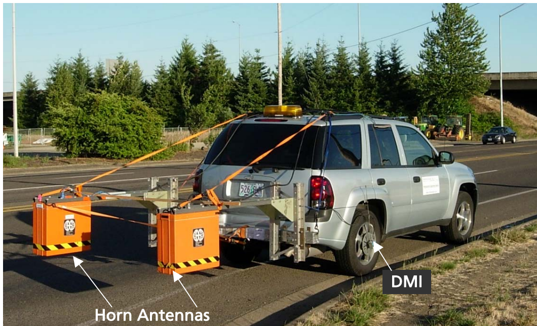
Figure 1 – Field Setup of GPR Equipment
