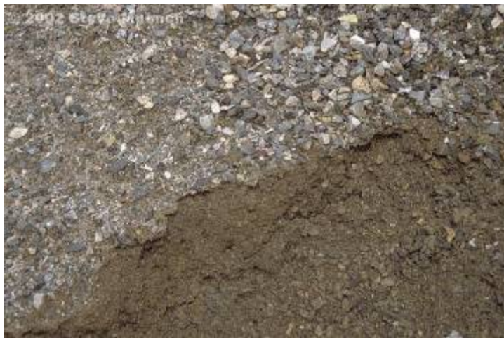
Figure A-5.4: Aggregate Segregation in Stockpile ( After WAPA 2002 )
