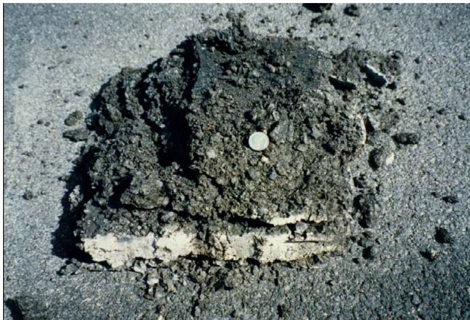
Figure A-3.2: Example of a Stripped HMA Mix (After Kandhal 2001)
