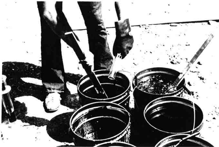
Figure 8. Adding initiator to resin.
