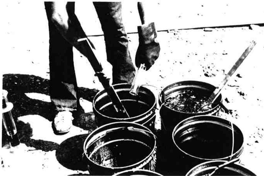
Figure 8. Adding initiator to resin.
