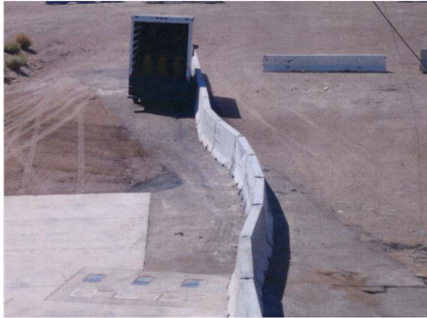
Figure 3.6: Tall F-shape barrier following Crash Test 3
