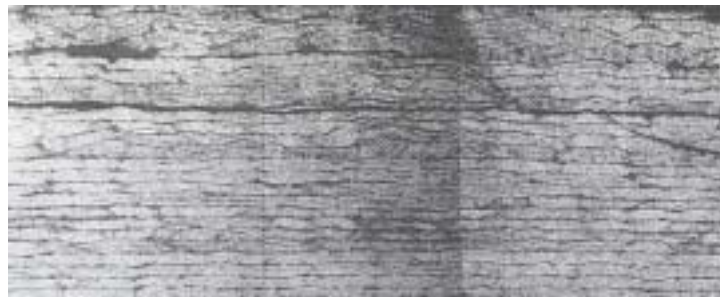
Figure 3-36: Microscopic View of Interlaminar Cracking
