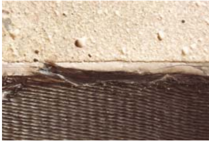
Figure 3-29: Pullout of Loose Fiber During Infiltration
