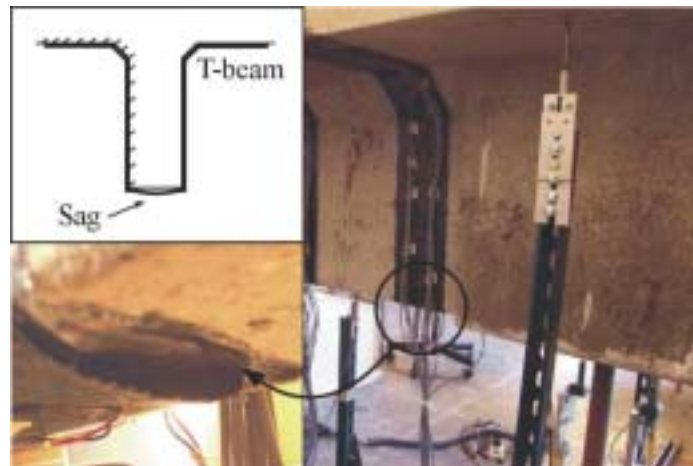
Figure 3-21: Sagging of Infiltrated Composite Material
