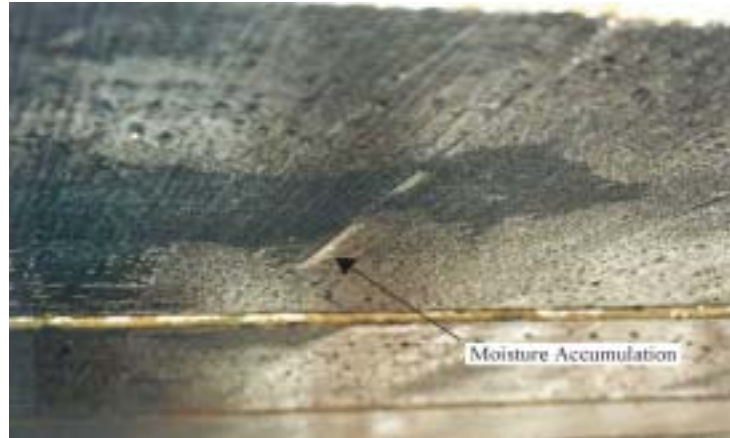
Figure 1-4: Delamination Due to Entrapped Moisture
