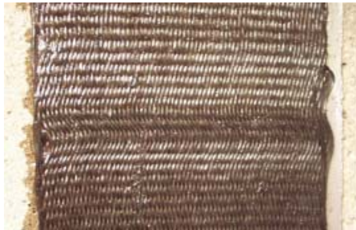
Figure 3-26: Waviness Caused by Improper Rolling
