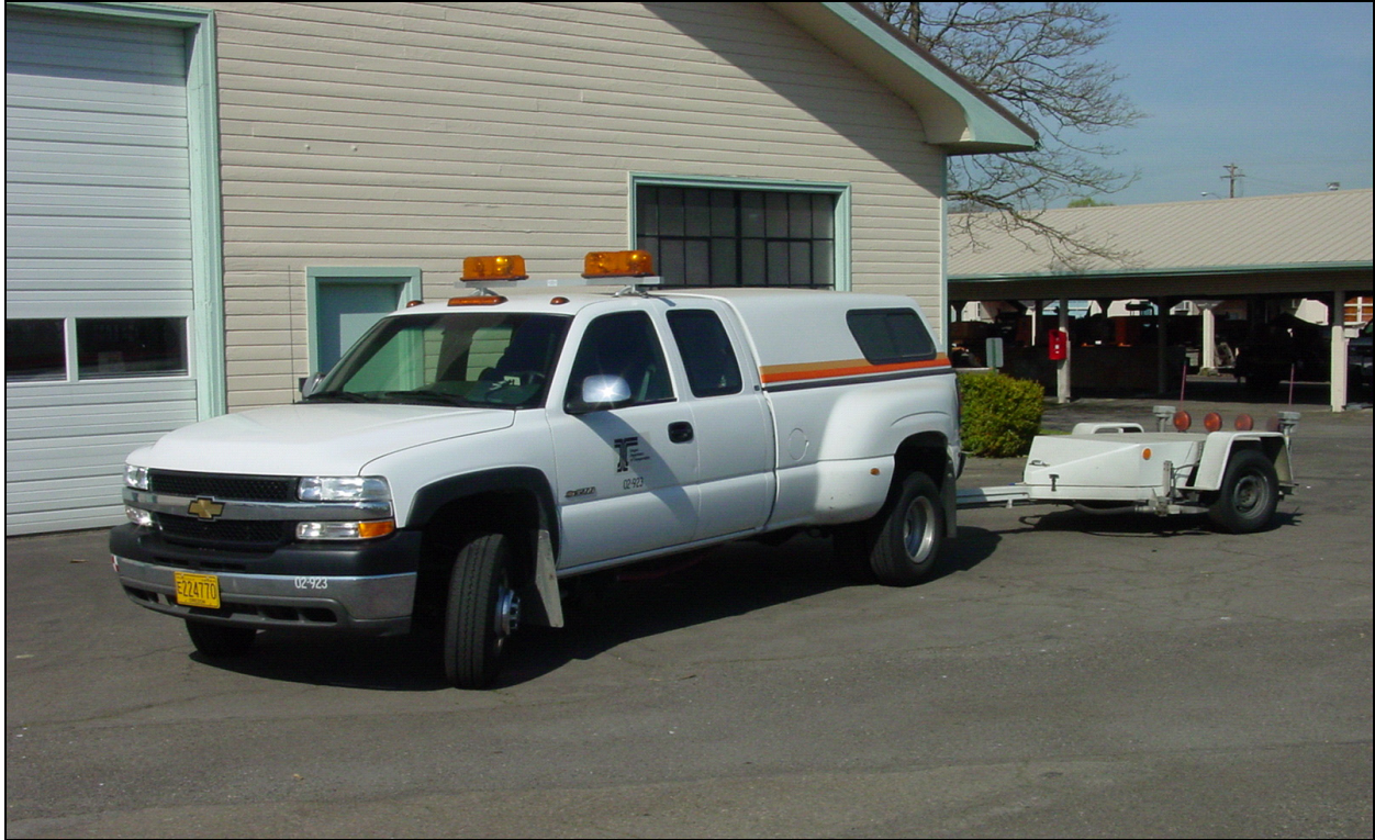
Figure 4.1: Tow truck and skid test trailer
