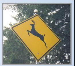
One less than ideal aspect of the experiment was the lower than desired strength of the strobe lights (more powerful solar strobes were available, but at a higher cost). While the flash was visible at the top of the deer sign from 0.6 mile, a stronger flash might have better attracted driver's attention.
