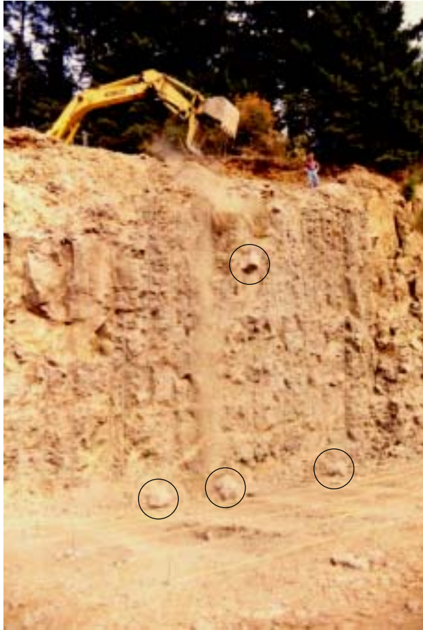
Figure 3.3: Rockfall testing; 12.2-meter high vertical presplit slope, 0.6-meter diameter rocks, 1V:4H catchment area foreslope. Circles denote test rocks.
