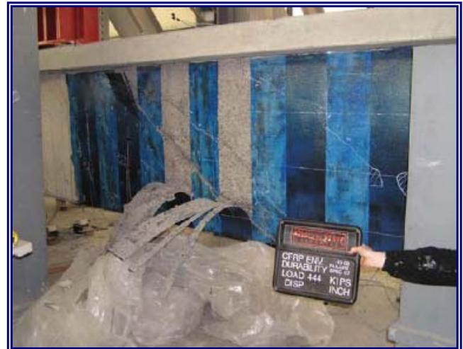
The research showed that conditions that allow moisture to get under the CFRP combined with freeze-thaw were detrimental to durability. In addition, the results showed that the American Concrete Institute (ACI) design code for CFRP did not provide a consistent level of safety for environmental exposure conditions. Consequently, the research provided design calculations to account for possible degradation
