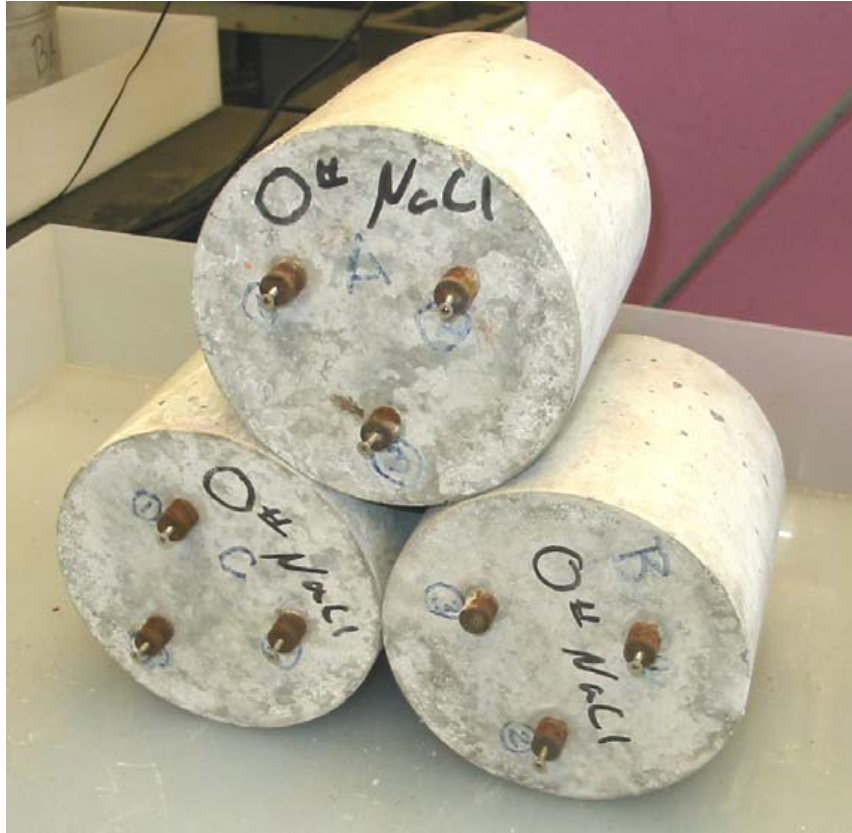
Figure 3.1: Three steel electrodes embedded in each concrete cylinder for measurement of corrosion rates by various instruments (CRMDs) and techniques as a function of chloride concentration in the concrete.
