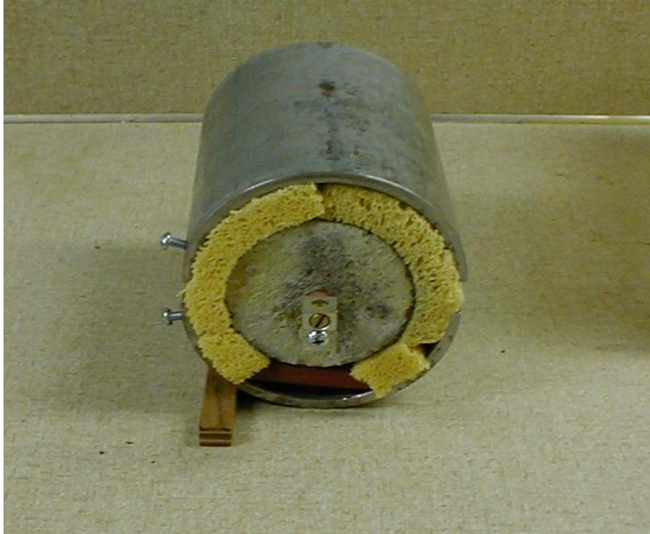
Figure 3.2: A steel electrode embedded in chloride-containing concrete cylinder for cyclic measurement of rebar polarization. The concrete cylinder is surrounded by a galvanized steel shell used as the counter electrode and moist sponges to act as the electrolyte.
