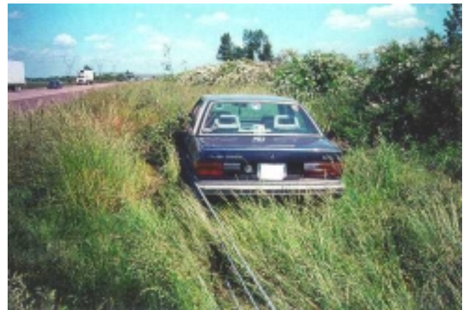
Vehicle prevented from crossing into oncoming traffic.
