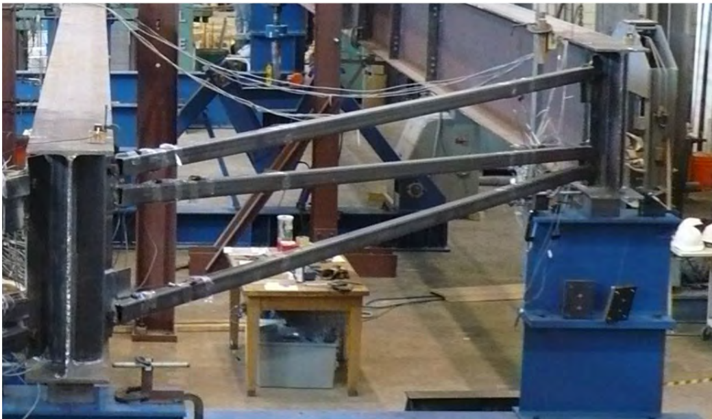
Figure 3.34: Split pipe end cross-frame (SE cross-frame shown)
