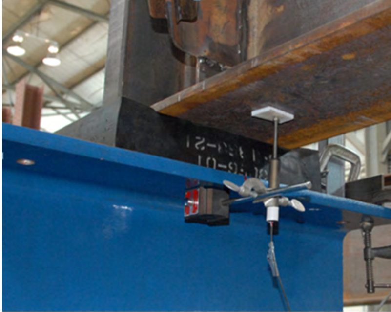
Figure 3.59: Measurement of bearing pad deformation
