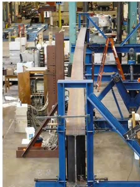
Figure 3.23: Typical single girder lateral load test
