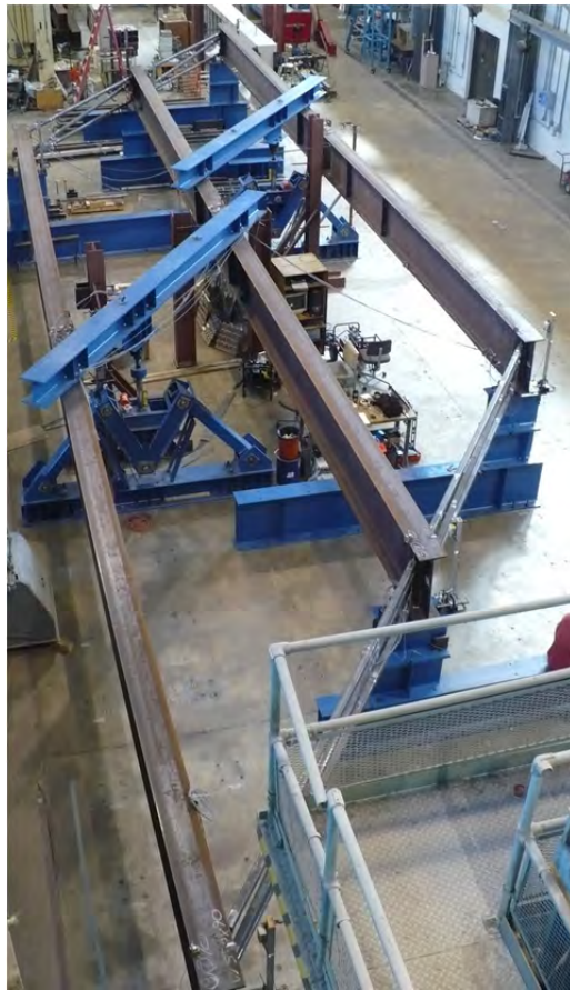
Figure 3.31: Three girder test (53° skew and no intermediate frames- looking south)
