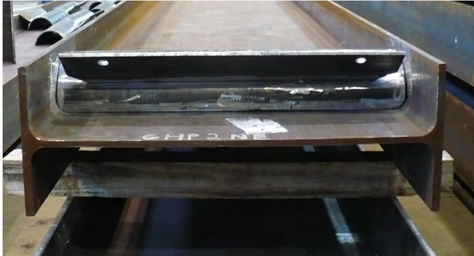
Figure 3.14: Split pipe stiffener prepared for welding
