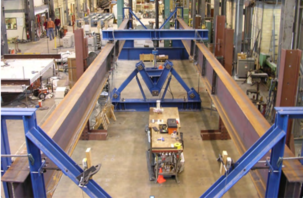
Figure 3.15: Twin girder buckling test (looking north)
