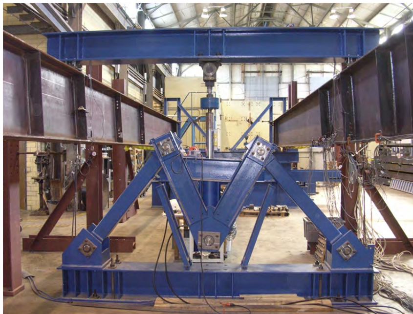
Figure 3.18: Gravity load simulator applying vertical load (looking south)
