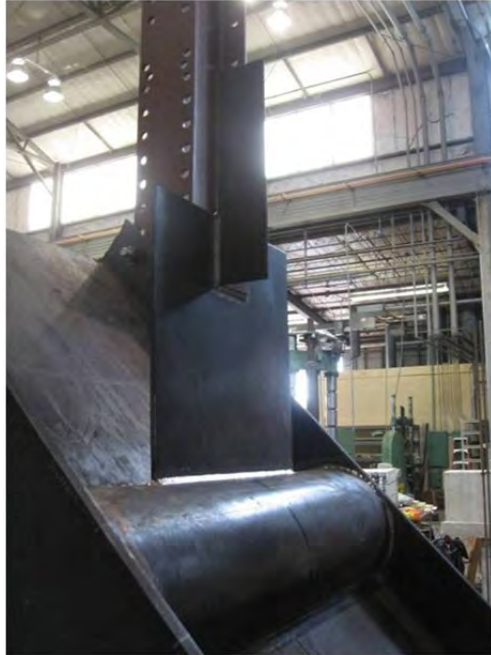
Figure 3.3: 45° Split pipe connection specimen
