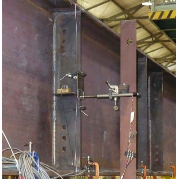
Figure 3.21 Lateral load test instrumentation
