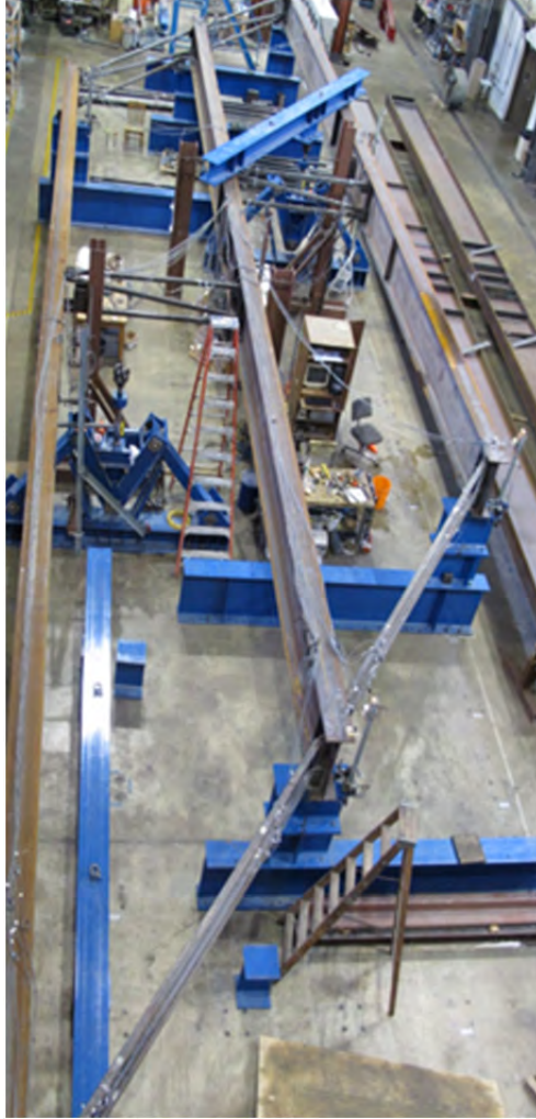
Figure 3.55: 53° Skew GBP specimen with staggered intermediate cross-frames, partially loaded
