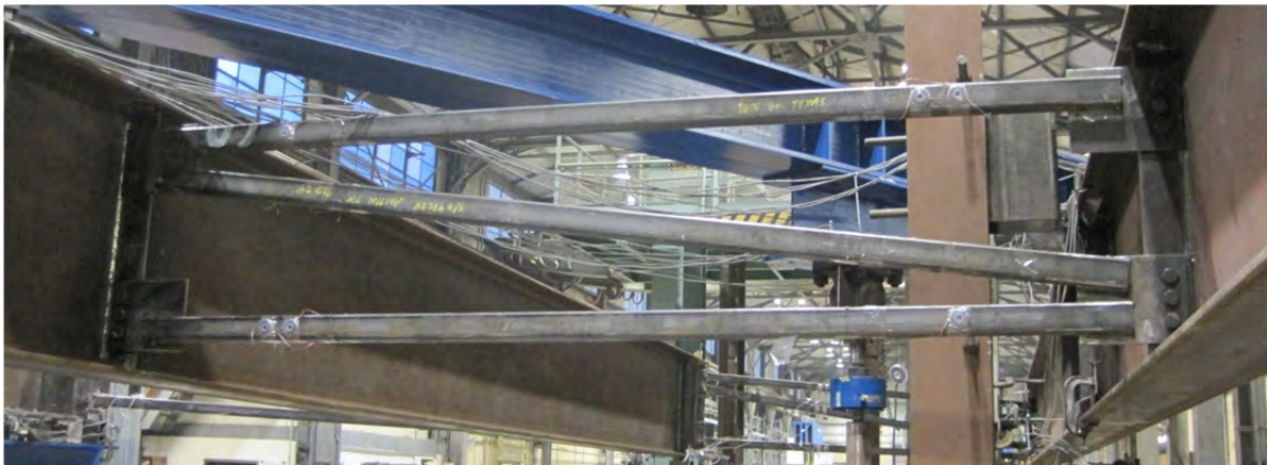
Figure 3.36: Intermediate cross-frame (western frame shown)
