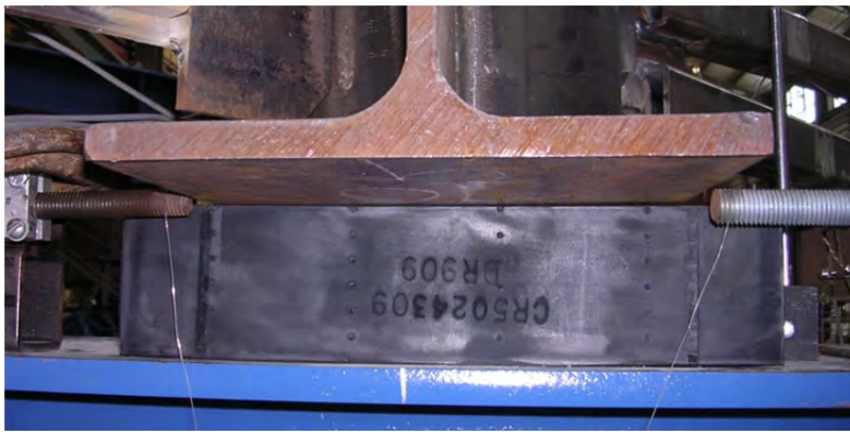
Figure 3.58: Rubber bearing pad with shims
