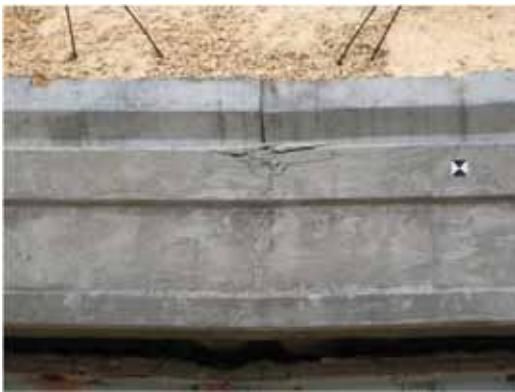
(c) Railing crushing from top
