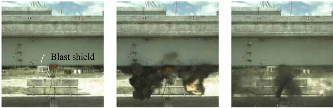
Figure 5.2: 1st bridge fracture test (bottom flange removal by explosion)
