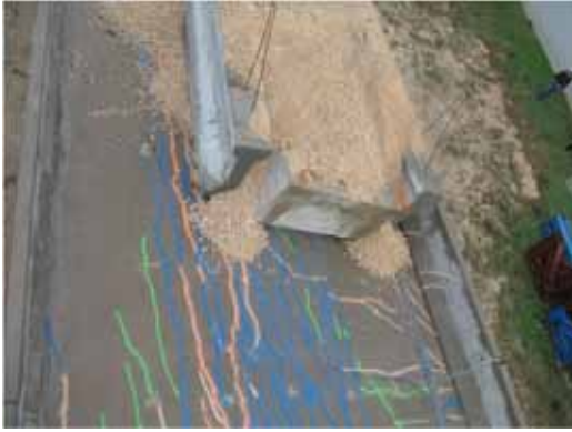
(a) Tensile cracking on top of the deck above IG-In top flange
