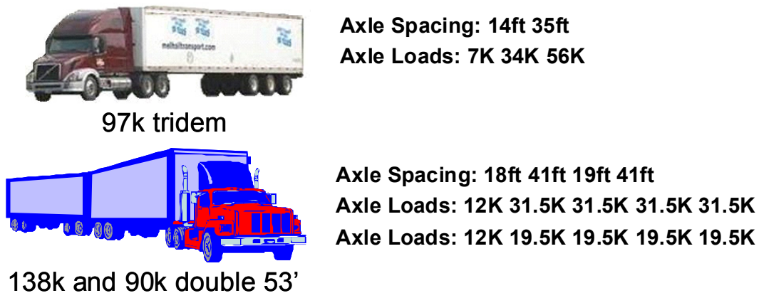
Figure 3.4: LCV Configurations for Bridge Analysis
