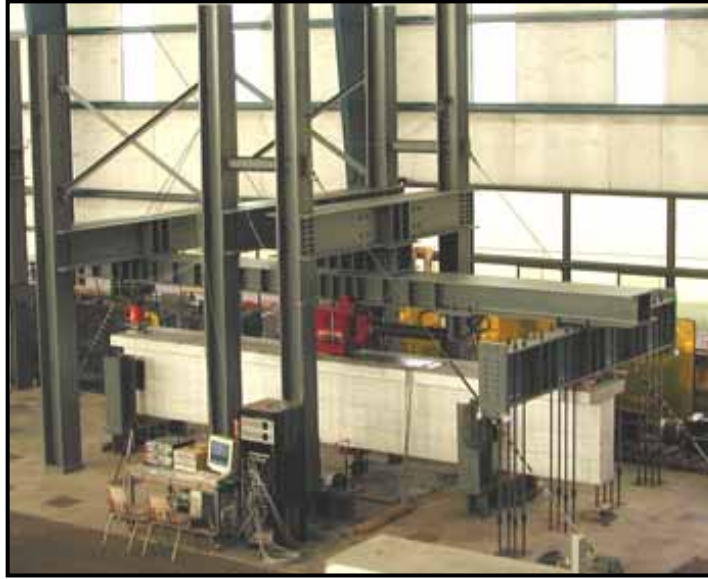
Moving load apparatus with cantilever supports
