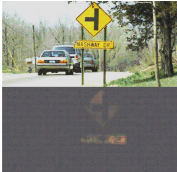
Retroreflectivity can affect the readability of signs at night, as shown in comparing the bottom photo with the top. (Source: FHWA)
