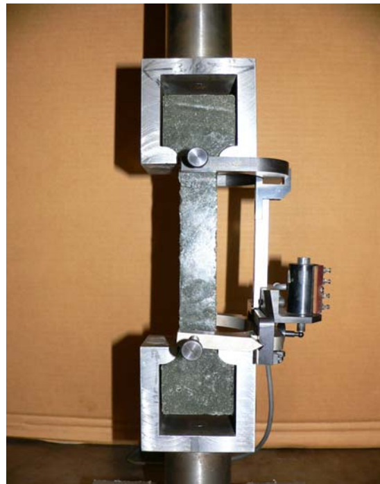
Testing wearing surface material
