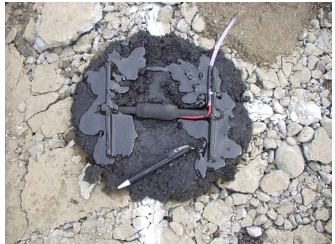
Strain gage on build-up of mastic mix over the rubbilized concrete base
