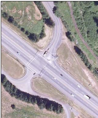
Traffic signal has good visibility from both major approaches
