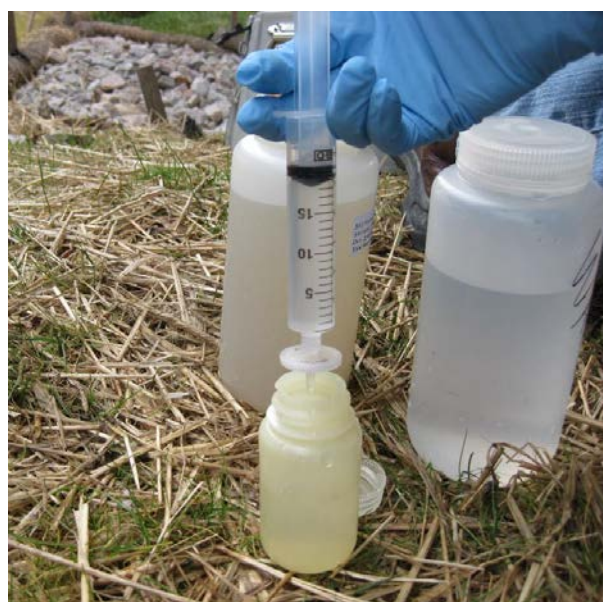
Figure 9. Filtration of water sample for dissolved metals.
