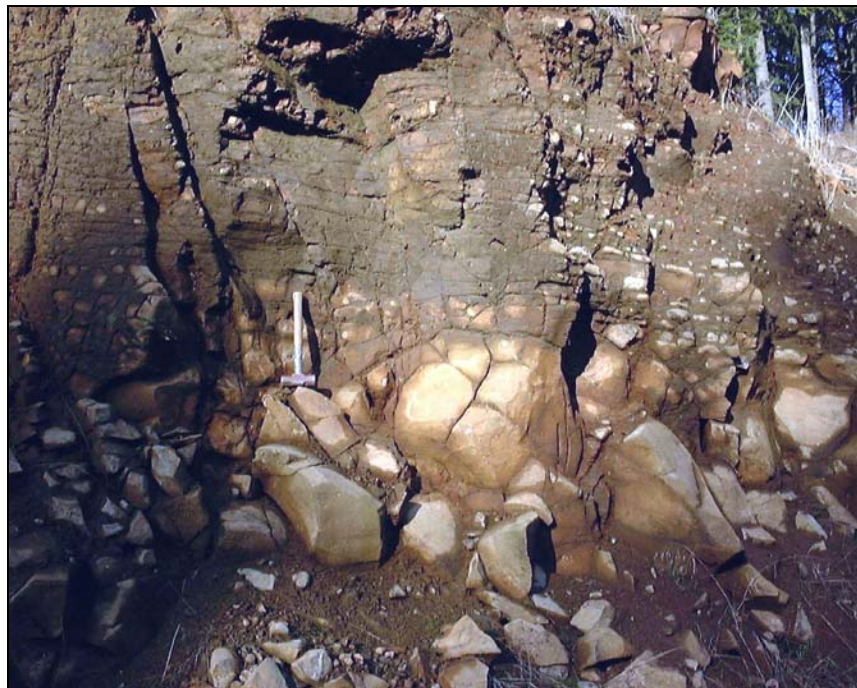
Close-up view of the basalt showing the weathered horizon and the fracture pattern.
