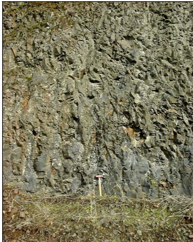
Close-up view of the jointing pattern, with 4lb. maul for scale.
