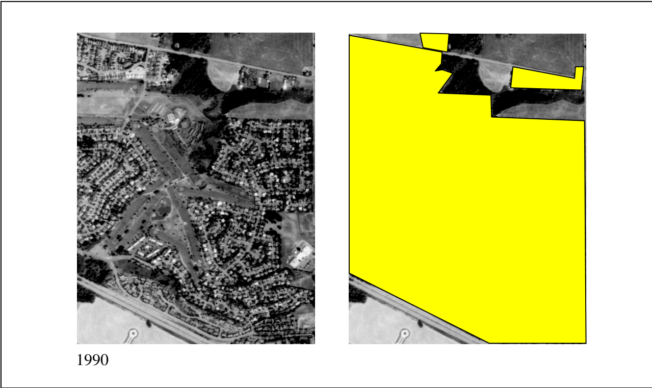
Figure C.6: Step 4. The Boundaries of Developed Areas are Digitized for the 1990 Aerial Photos
