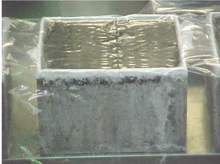
Figure 2.2: Concrete slab undergoing ponding
