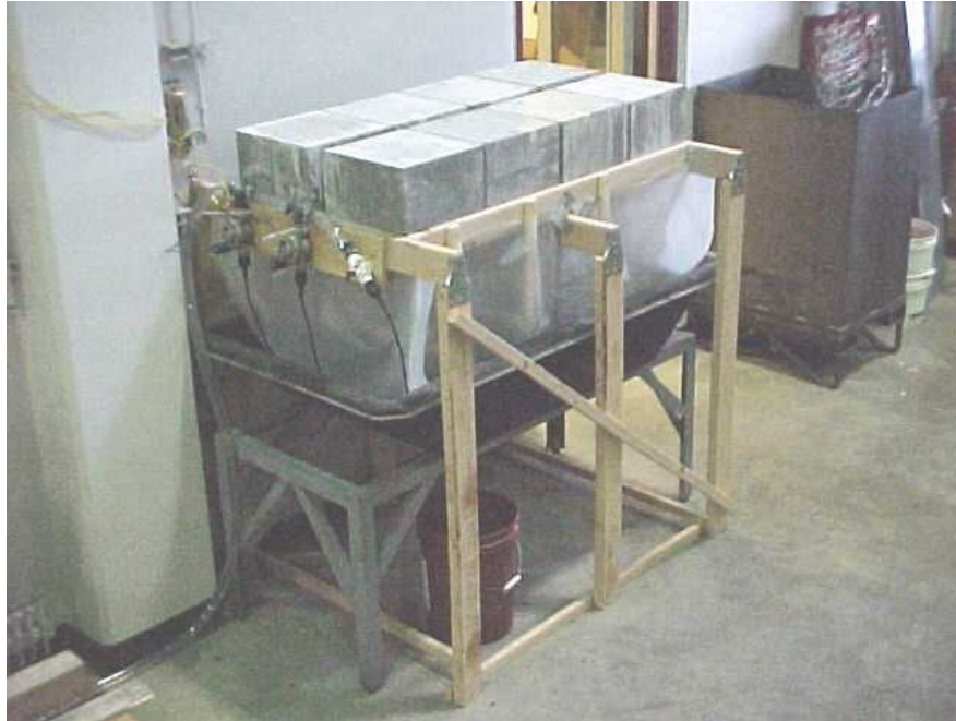
Figure 2.3: Rack for washing slabs
