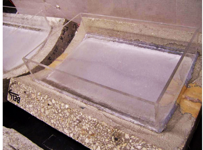
Experimental setup showing RCP section with induced crack of selected width. The test chamber for chloride exposure is fastened to the section with sealant.
