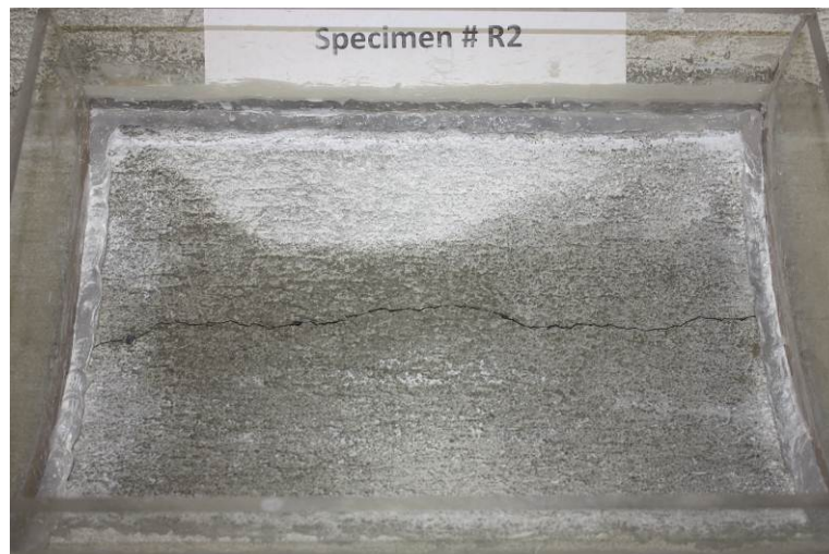
Figure (4.4) R-type specimen with 0.02-in-wide crack after exposure to saturated calcium hydroxide solution
