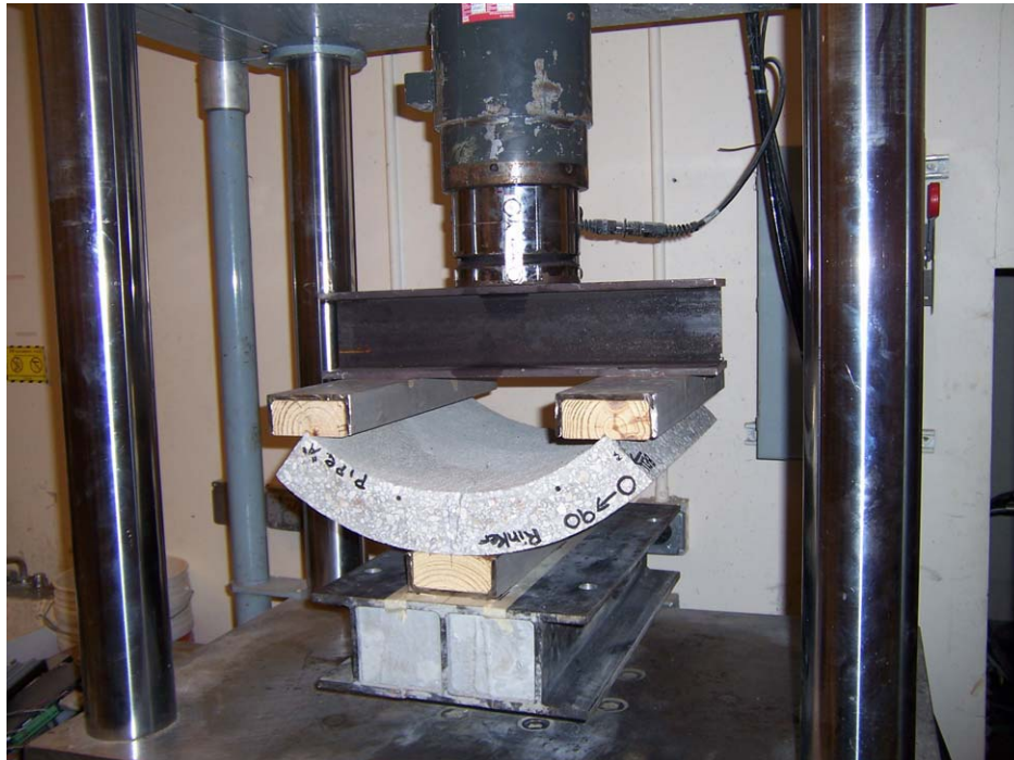
Figure (3.12) Cracking rig used to generate cracks in RC culvert pipe specimens
