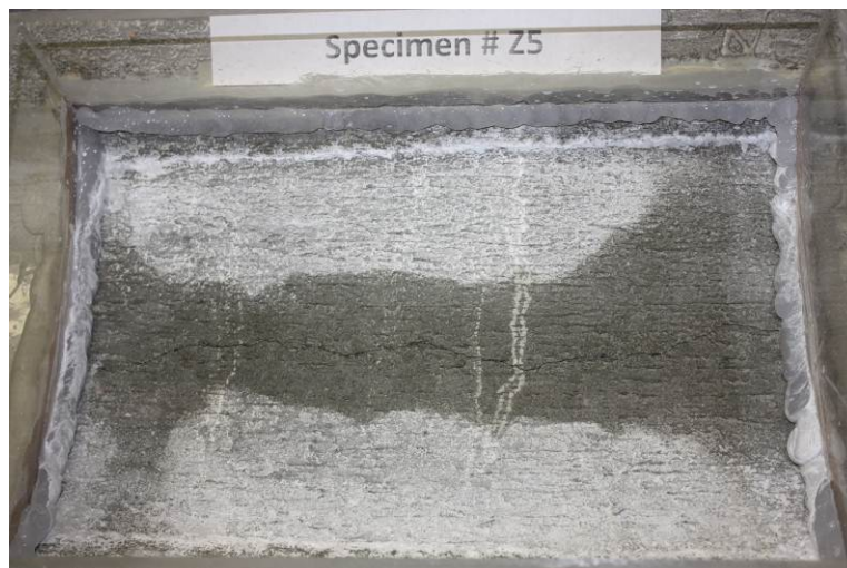
Figure (4.2) Z-type specimen with 0.02-in-wide crack after exposure to saturated calcium hydroxide solution
