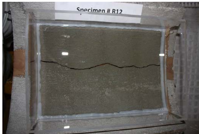
Figure (3.18) A cracked specimen during exposure to the chloride solution
