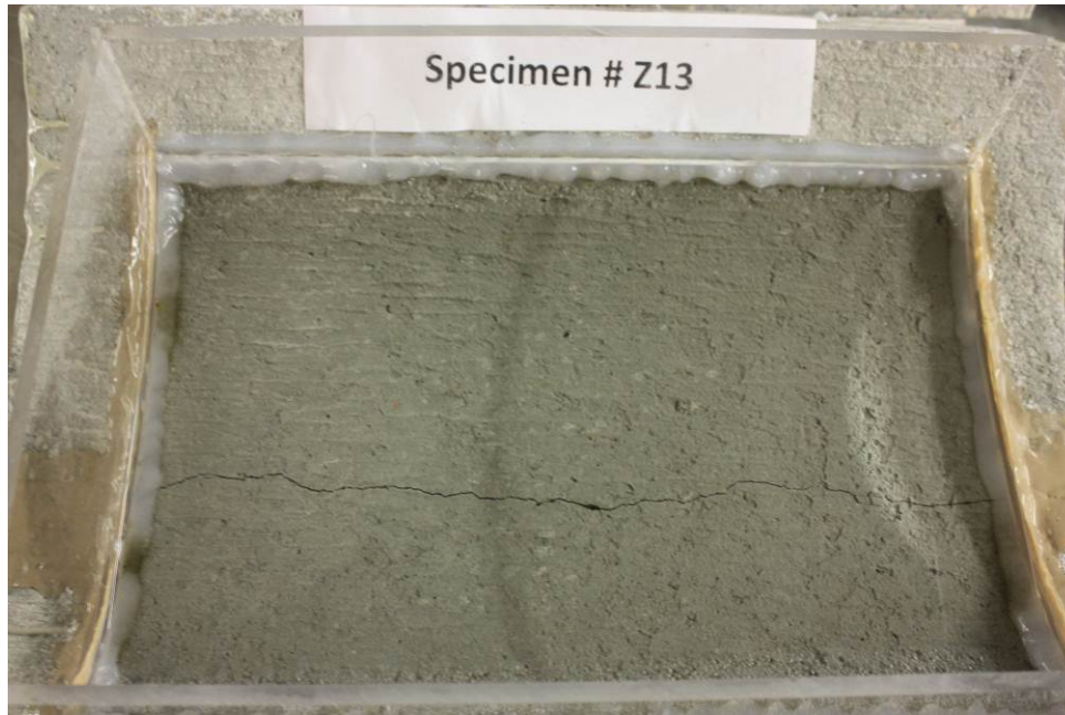
Figure (4.14) Specimen Z13 (0.020-in-wide crack class) showing no corrosion product spots about 52 days after the ponding solution started to incorporate chloride ion
