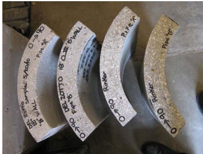
Figure (3.2) RC pipe specimens as received with FDOT identification
