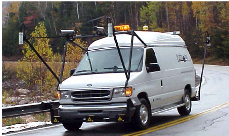
Figure 7. Pavement distress data collection van (Pathway 2008).
