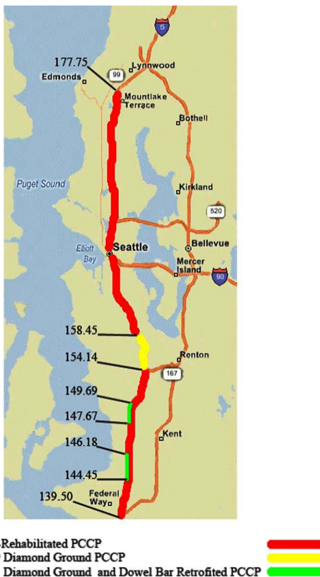
Figure 5. Rehabilitation of PCC pavement on I-5 in King County as of 2004 (from Hansen et al. 2007).
