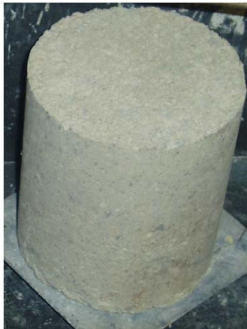
Figure 1 Cement stabilized limestone screenings
